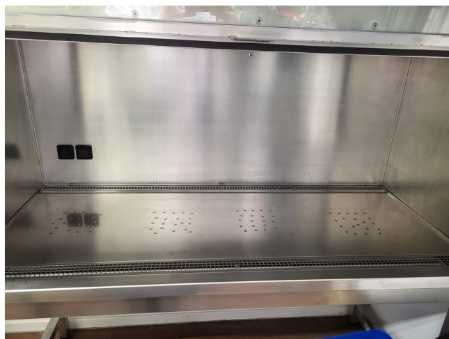
FIGURE 1 | Illustration of the sampling strategy, wherein a stainless-steel surface was divided into four areas, each measuring 20 by 20 cm (400 cm 2 ), labeled as Areas W, X, Y, and Z. Each area was spiked with 1 mL of an acetonitrile–water mixture (1:1, v/v) or 1 mL of solution containing different concentrations of a mixture of HMPs (Solution W, X, Y, or Z). The 1-mL volume was evenly distributed across each area in the form of 20 small drops.
